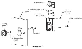
3. Fix the striking plate by screw ST3.5X18 (Make sure latch works well)
