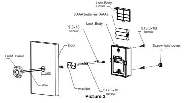
3. Fix the striking plate by screw ST3.5X18 (Make sure latch works well)
